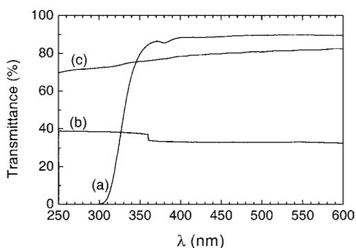
Figure 2 Transmittance spectra for microscope slab glass (a), aluminum polyphosphate compact (b), and a quartz slab (c).
