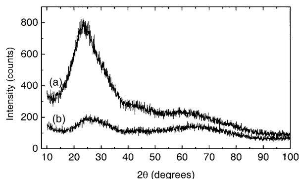
Figure 1 Typical X-ray diffraction patterns for powder sample (a) and compacted sample (b).
